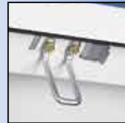
ZINC PLATED LATCH STRIKERS (1/4" ROD) BOLT SECURELY TO COVER SUPPORT CHANNEL WHICH IS REINFORCED IN THE LATCH STRIKER AREA
